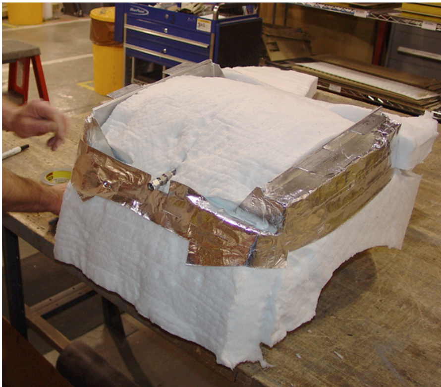
Figure 19. Taping Down the Insulation (Sheet 1 of 2).
