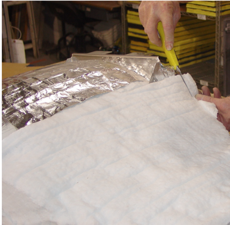
Figure 21. Trimming Insulation from Plenum (Sheet 1 of 2).
