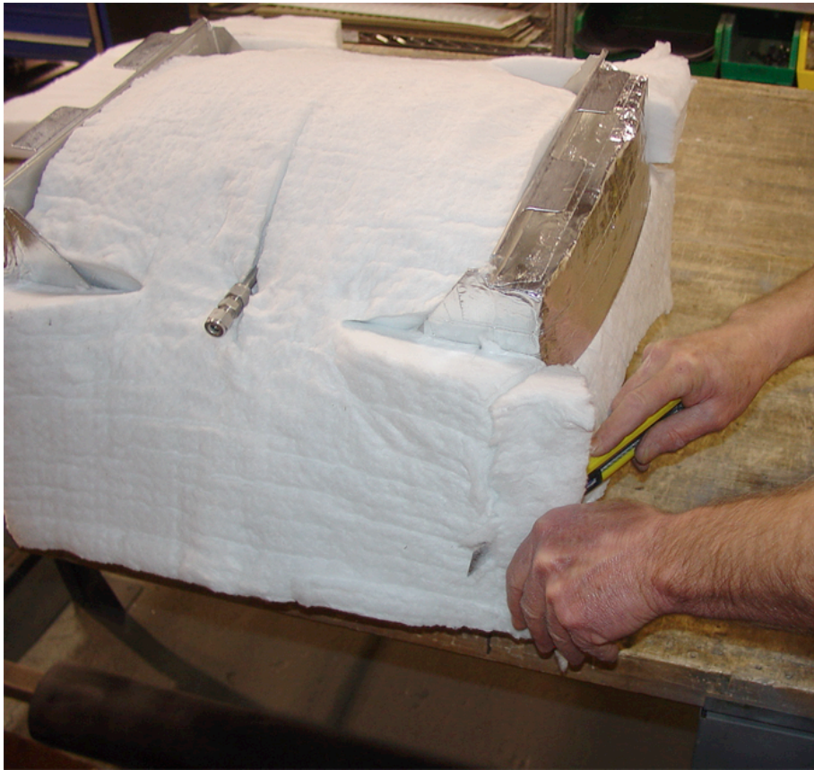
Figure 18. Trimming Insulation on the Plenum (Sheet 1 of 2).
