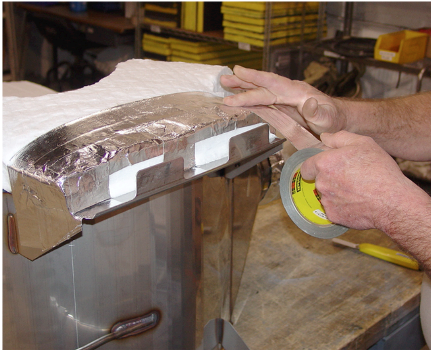
Figure 13. Wrapping of the Plenum.
