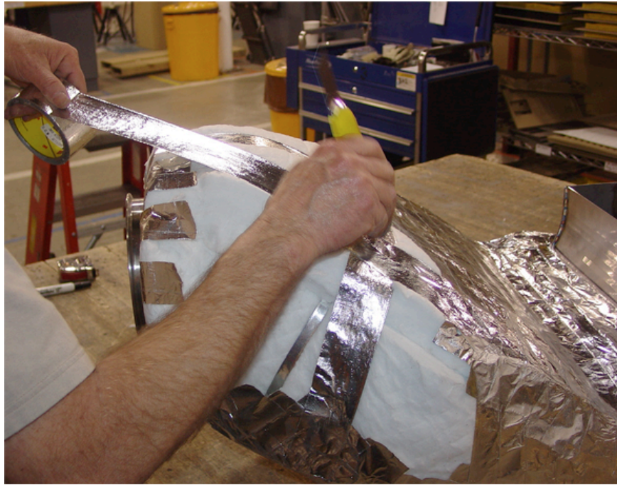
Figure 33. Taping the Top Portion of the Plenum.
