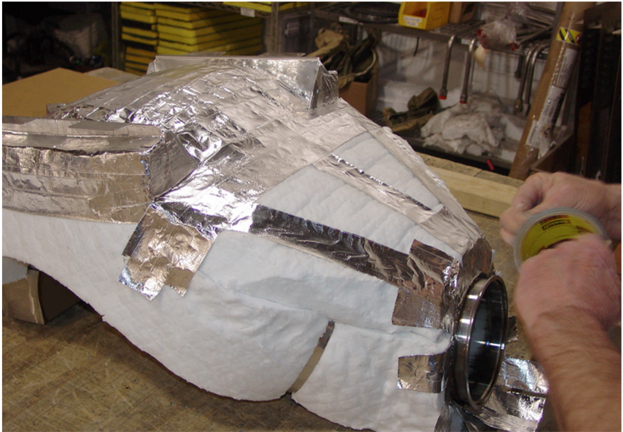
Figure 24. Insulating the Top Snug (Sheet 1 of 2).
