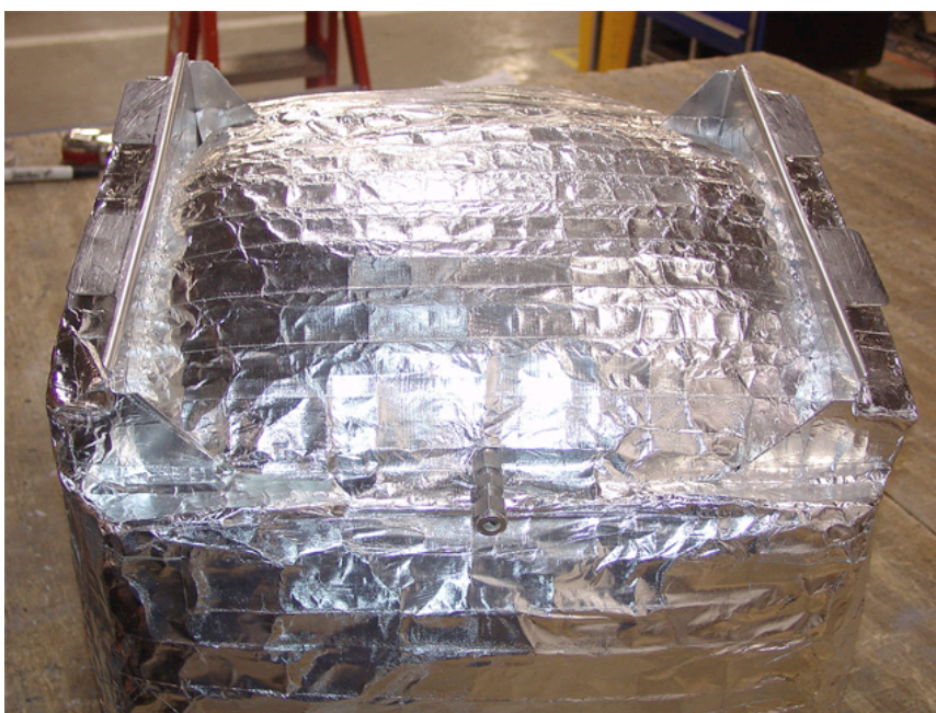
Figure 20. Taping Down the Insulation Around the Extension Tube (Sheet 3 of 3).
