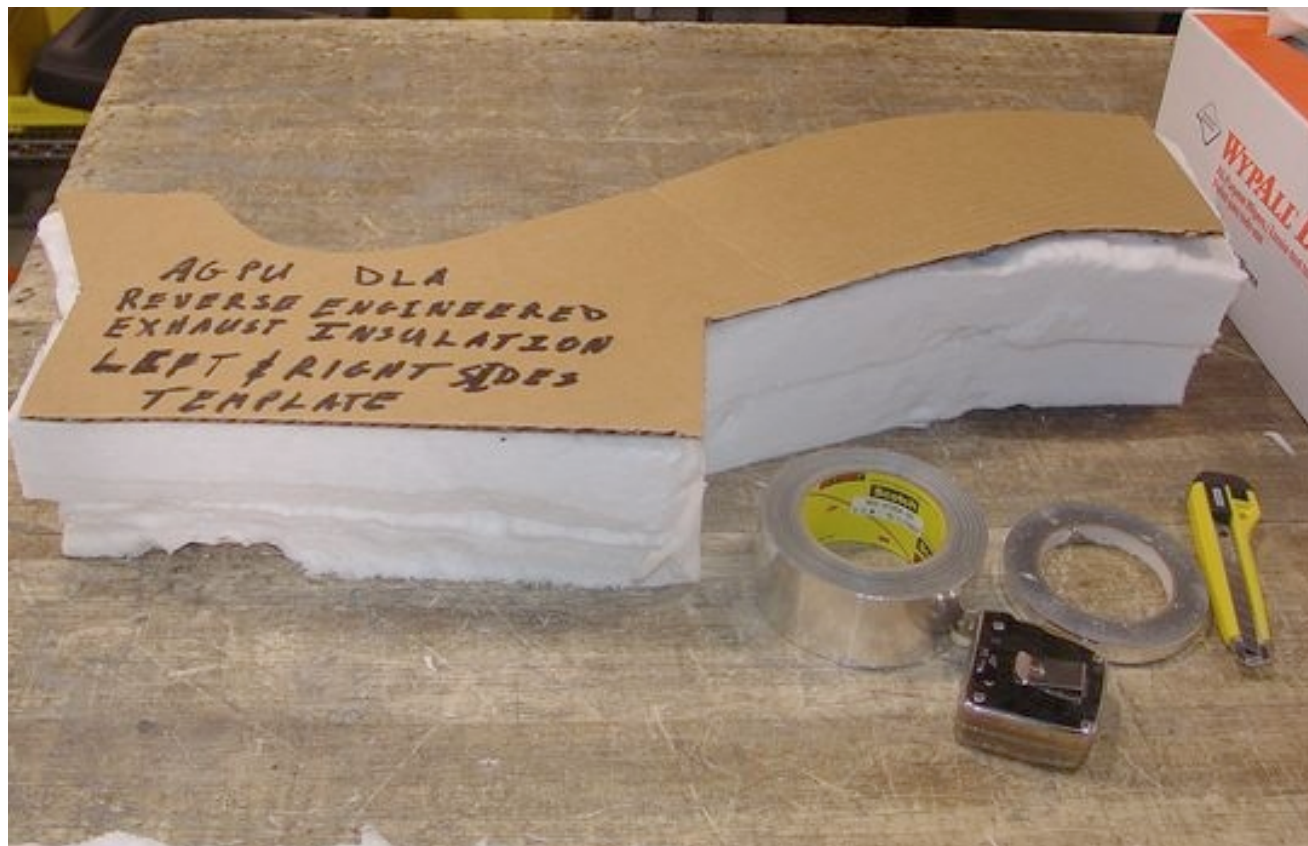
Figure 6. Plenum Template (Sheet 2 of 3).
